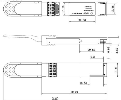
Figure 10. Mechanical Specifications
