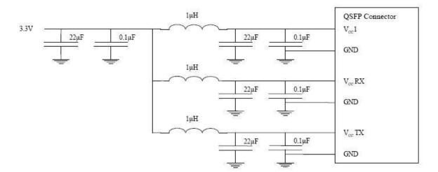
Figure 3. Host Board Power Supply Filtering
