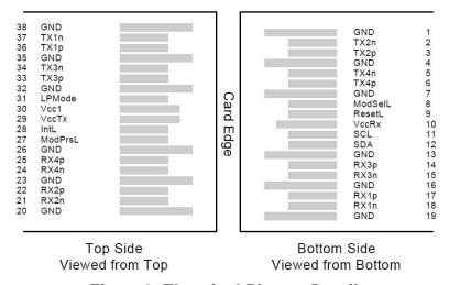
Figure 2. Electrical Pin-out Details
